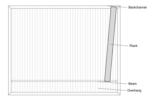
Planks running parallel with the roof sheets, without others planks at 90 degrees, should be angled over atleast 2 roofsheets and extend to within 200mm of the backchannel or beams but preferably over them.
